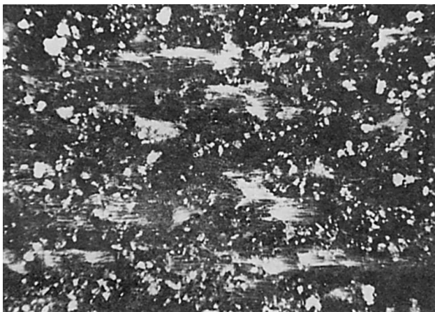
Fig. 18. Photomicrograph of the fractured surface from joints with the highest fracture energy. Observe wood failure. White circular areas represent fillers (walnut shell flour). Note distinct fibrous structure (wood) soaked in adhesive (dark). Each fibrous structure terminates on the fractured surface with whitish area and indicates that the locus of failure occurred in the wood immediately surrounding the adhesive-soaked wood.
