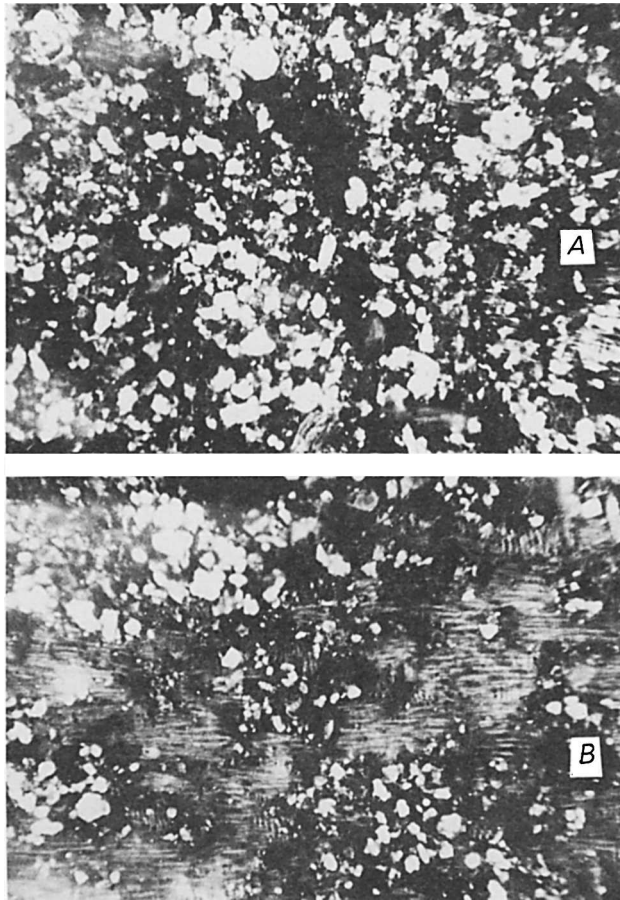
Fig. 19. Relative abundance of fillers (white areas) on the fractured surfaces of the opposing sides of the two adherends in a joint. Crack growth appears to have occurred by failure in adhesion between fillers and the adhesive.
